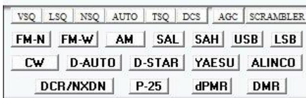
If you 'right-click' the VSQ (Voice Squelch) button, a window appears and you can use the sliders to adjust the 'Squelch Level' and 'Delay'.
